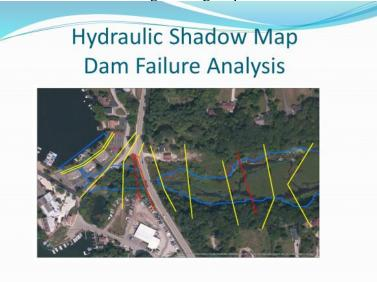
One of the requirements for us recently, was to complete a study showing the areas that would flood should our dam or an embankment give way. Walworth County will then apply appropriate zoning to the area.
